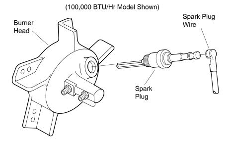
Figure 9 - Spark Plug Removal
